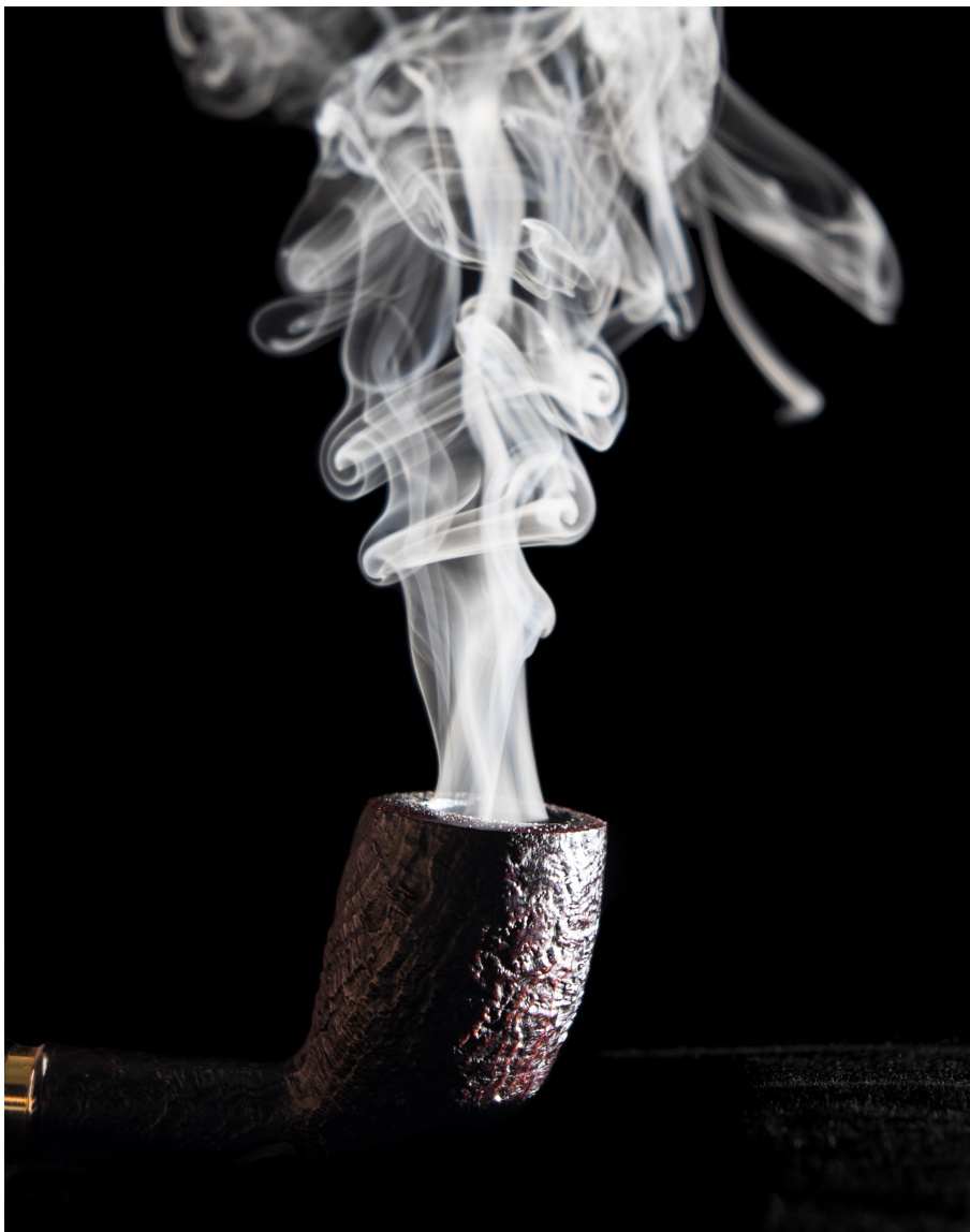
Figure 1.1: Plume of smoke rising from a pipe. The picture illustrates different flow regimes: laminar (close to the pipe), transitional (at the height of the vortex rings), and turbulent (towards the top of the frame). Own photograph.
